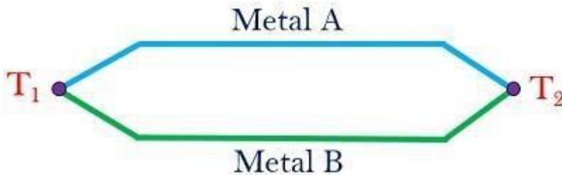
Seebeck effect states that when two wires of dissimilar metals form an electric circuit on joining, then current flows through that circuit if there exists a temperature difference between the two junctions.
