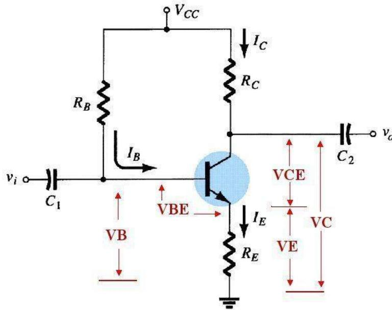
Applying KVL to the BE loop in clockwise direction
