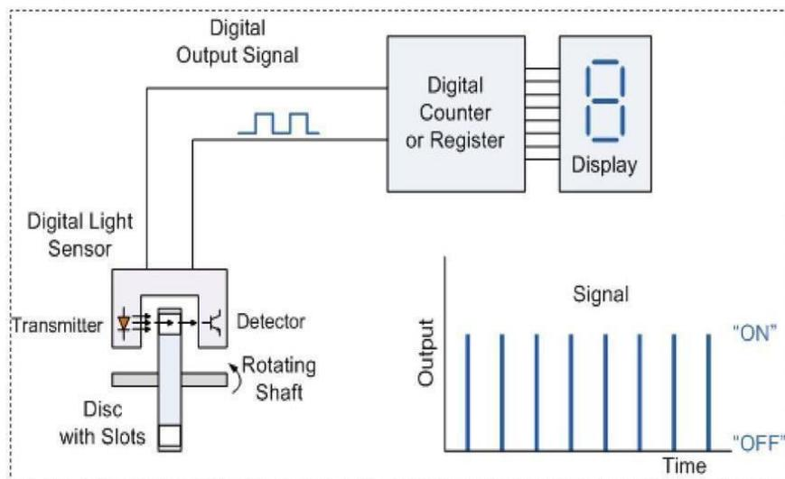
The following setup uses a light sensor to measure the speed and produces a digital signal.
