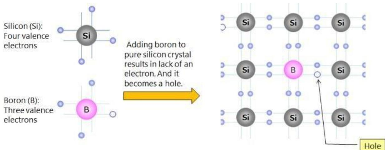
When P.D is applied to a P-type S.C the majority carriers of a P-type S.C i.e. holes which are +ve.
