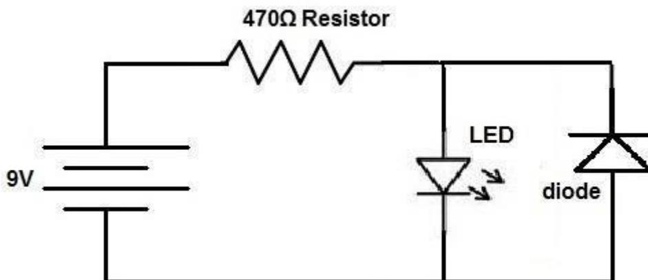
When reverse voltage greater than 3v is applied to a LED, the LED may be destroyed.
