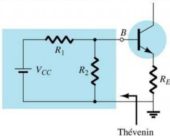
RTH:- Voltage source is replaced by a short circuit equivalent.
