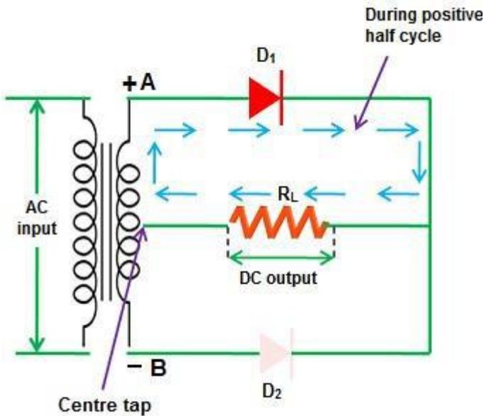
During the –ve half cycle of the input voltage, end A becomes –ve & end B becomes +ve.
