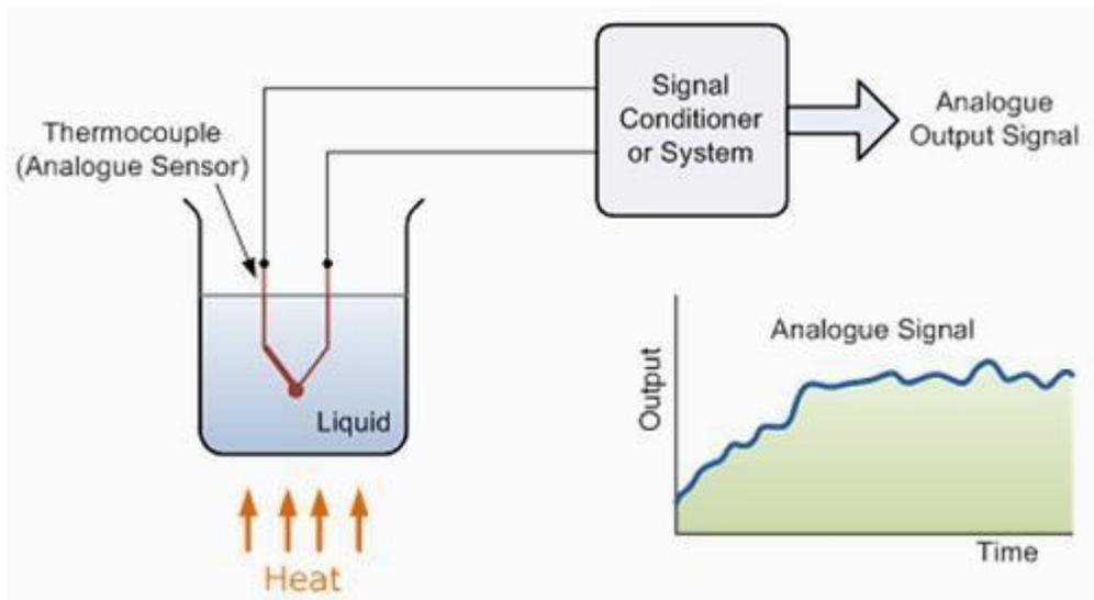
A thermocouple or a thermometer is an analog sensor. The following setup is used to measure the temperature of the liquid in the container using a thermocouple. The output of an analogue sensor tends to change smoothly and continuously over time.
