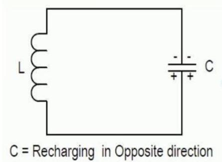
The collapsing magnetic field then recharges the capacitor due to which current now flows in opposite direction.
