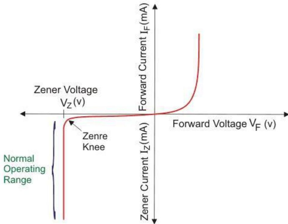
The above diagram shows the V-I characteristics of a Zener diode.
