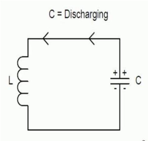
When the capacitor is fully discharged, the magnetic field begins to collapse thereby producing counter emf. Due to this emf the capacitor is now charged with opposite polarity, making upper plate -ve & lower plate of capacitor +ve.
