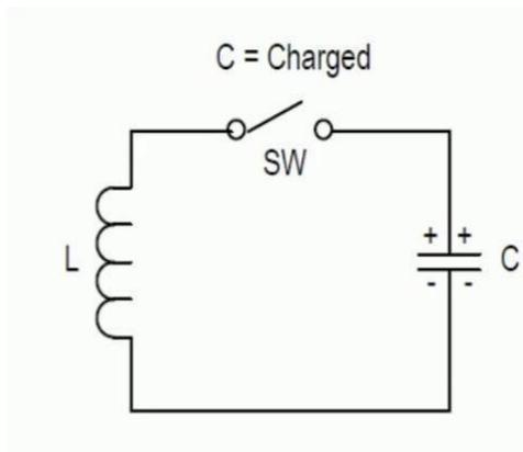
In the above fig. It is clear that the capacitor is charged from dc source and has electrostatic energy.
