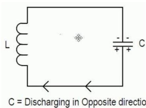
This continuous charging & discharging produces oscillatory current. The resonant frequency of the tank ckt. is given by,
