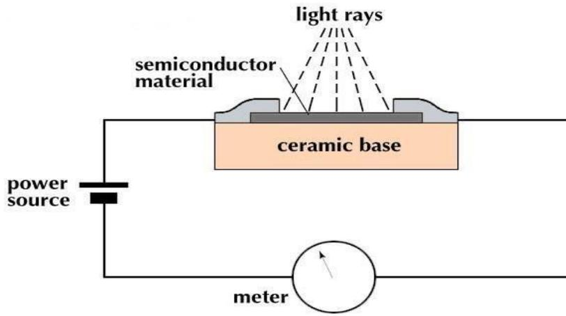
The resistance of the photoconductive material change when a beam of light is incident on it.
