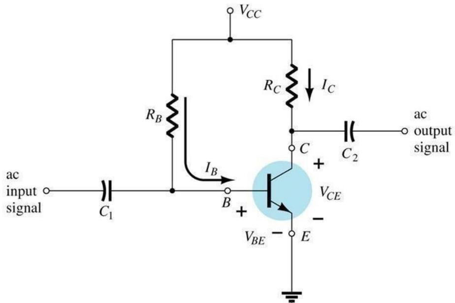
Applying KVL to the BE loop in clockwise direction
