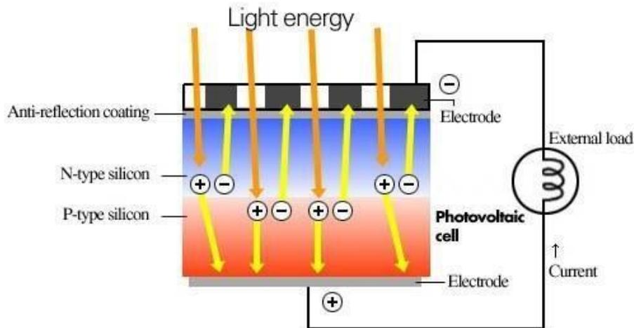
A P-type silicon and N-type material are diffused to form a photovoltaic cell. Silicon and selenium are used as a semiconductor material.
