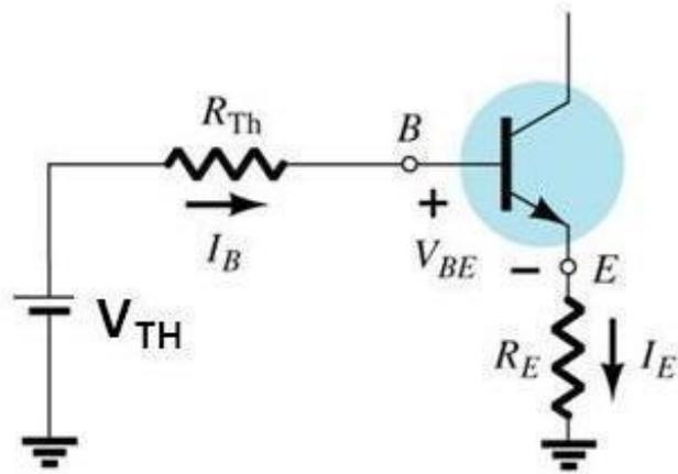
Inserting the Thevenin equivalent circuit
