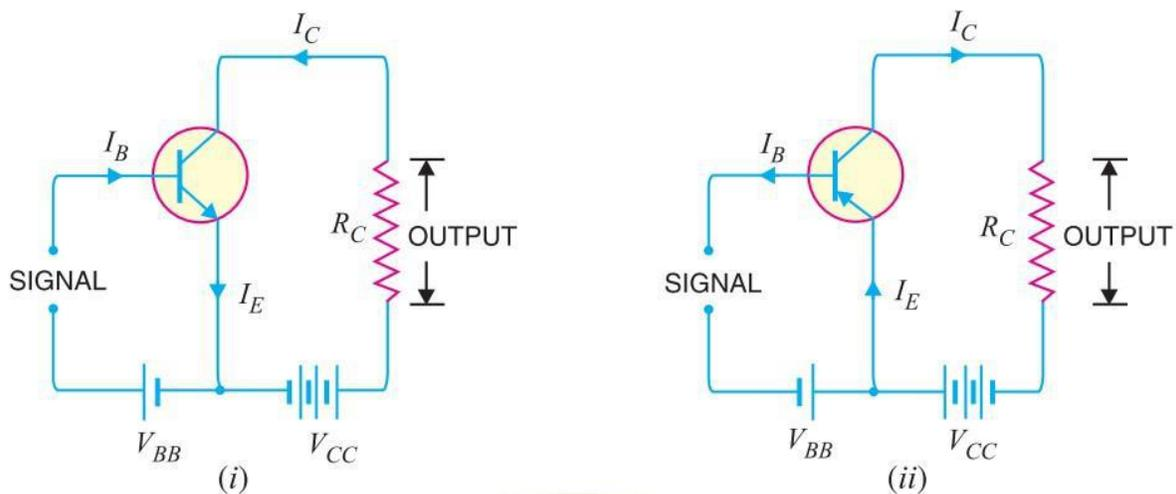
In the above circuit arrangement, input is applied between base & emitter & output is obtained from collector & emitter.
