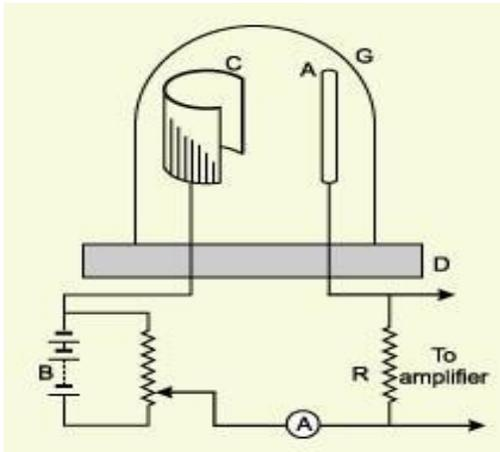
When a beam of light falls on the cathode, electrons are released from it, which are drawn towards the anode.
