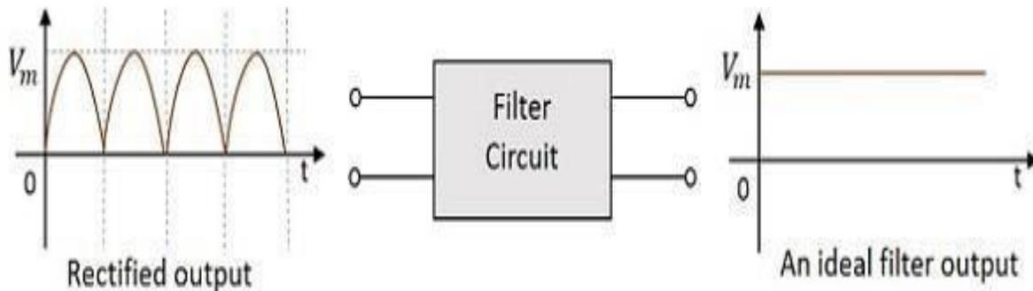
Filter circuits are classified into four types
