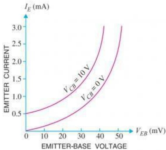
It is the curve between emitter current ( $I_E$ ) & base emitter voltage ( $V_{BE}$ ) at constant  $V_{CB}$ .
