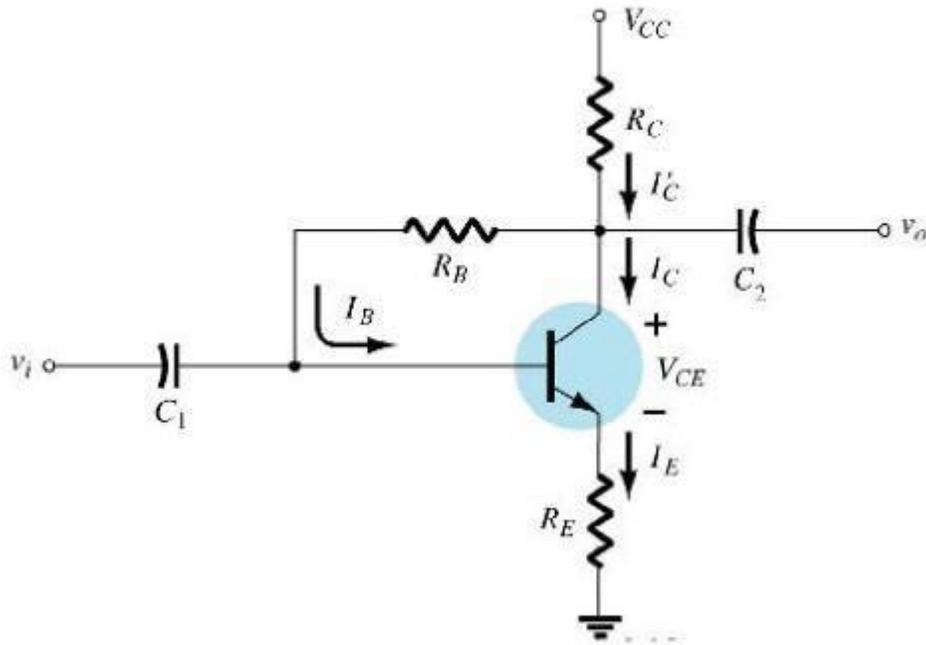
An improved level of stability can also be obtained by introducing a feedback path from collector to base.
