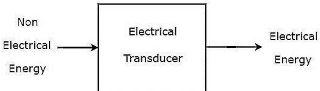
As shown in the figure, electrical transducer will produce an output, which has electrical energy. The output of electrical transducer is equivalent to the input, which has non-electrical energy.
