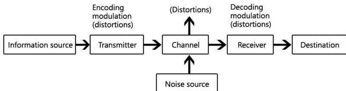
**Transmitter** - couples the message onto the channel using high frequency signals
