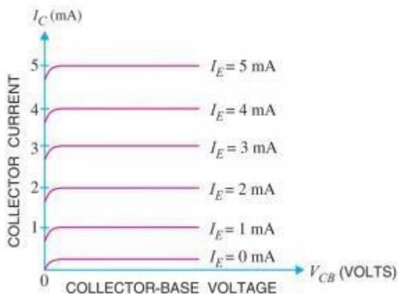
It is the curve between  $I_C$  &  $V_{CB}$  At constant  $I_E$ .
