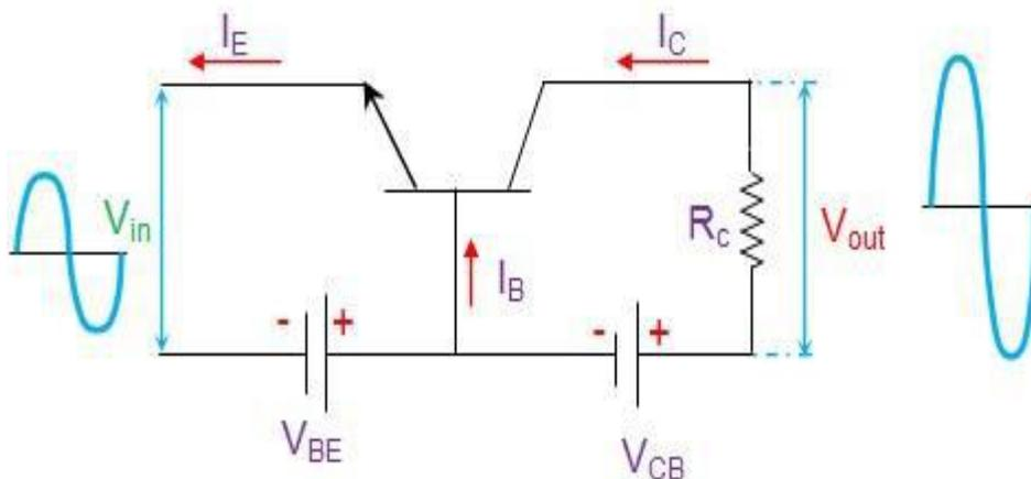
A weak signal is applied between BE junction & output is obtained across load  $R_C$ .
