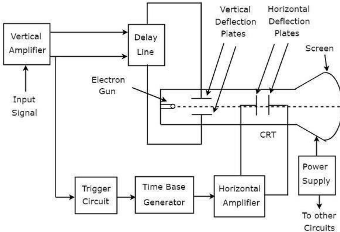
An oscilloscope consists of the following parts:
