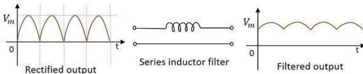
Hence, due to the presence of that leakage A.C component the output is pulsating one which can be removed by using more number of filter stages or by adjusting the component values.
