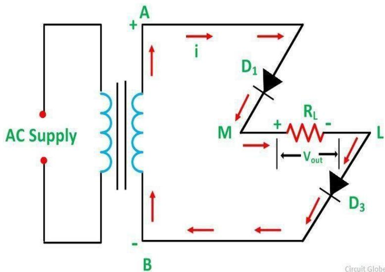
During the -ve half cycle of input voltage, end A becomes -ve & end B becomes +ve.
